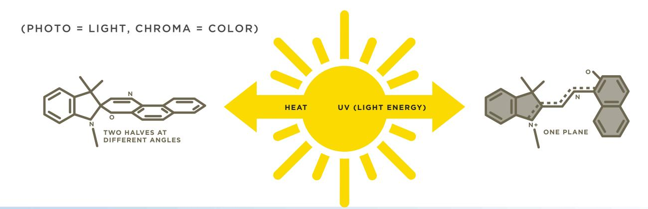
Photochromic technology has been a core competency at Transitions Optical for more than 25 years. The definition of photochromics is a light-induced, reversible change in color. A photochromic lens contains millions of photochromic molecules.
